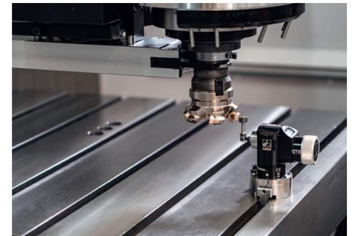
Radio table touch probe for tool measurement and tool breakage control. Including quick-change system.
